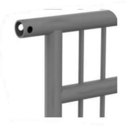
A unique anti-shock and anti-noise system! Ein einzigartiges Anti-Schock- und Anti-Lärm-System The panels of frontons and fences are made from an extremely rigid steel frame filled with solid round bars (diameter 10mm) passing through the horizontal tubes. This technique strengthens the grid (load capacity of 100kg/m) and makes it quieter (reduction of 78% in noise compared to solid panels).
